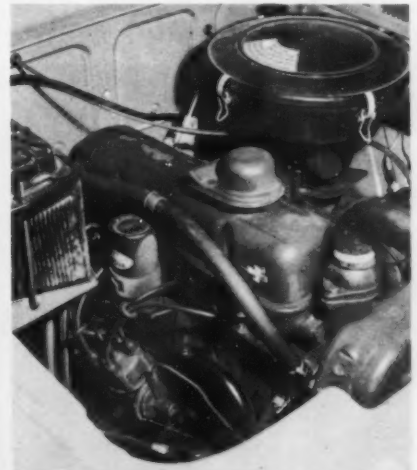
Unstressed, oversquare 1.5-ohv engine doesn't scream, should last a long time.
